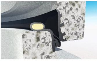
The **CSD-PLUS-3** can be combined with the integrated socket profile **MKP-97**, which additionally lines the sockets sealing surface.
